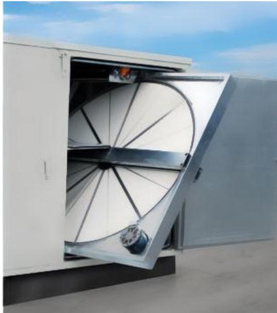
**Airxchange's** energy recovery ventilation wheel allowed the architect to reduce the required size of the school's packaged HVAC unit by half.
