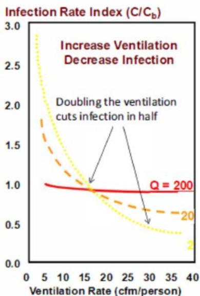
Exceeding minimum ventilation standards may be the most powerful means to reducing infection rates. Riley and Nardell (1989) present a standard model of airborne infection usually referred to as the Wells-Riley equation. Increasing ventilation rates decreases exposure by diluting air containing infectious particles with infectious-particle free air. Using the Wells-Riley equation, doubling ventilation rates has the potential to reduce infection rates by half.
