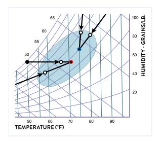
Airxchange wheels recycle energy to precondition ventilation air and reduce outdoor air loads up to 80%.
