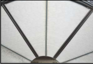
Figure 22 Embedded stiffener faces motor side.
