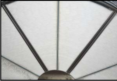
Figure 18 Embedded stiffener faces motor side.
